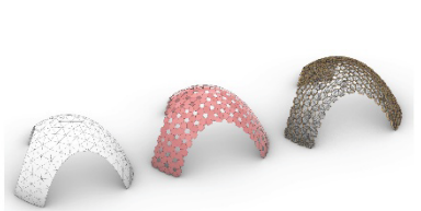
Second scenario: Doubly curved vaulted structure, necessitating the design of variable components. A solver that generated non-linear tessellations of planar hexagons was developed, ensuring planarity by inscribing each component within a triangle.
