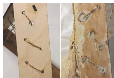
Detail of the plywood frame of the hyperbolic paraboloid panel, before and after the mycelium aggregation with the plywood.
